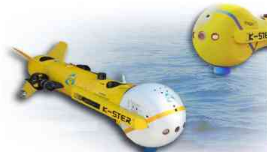
Picture 4 - Remote-controlled underwater vehicles K-Ster With a mine search and destruction system
